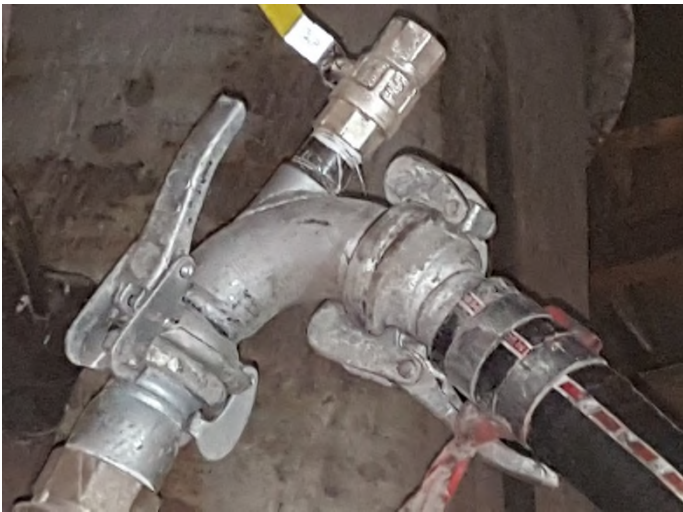
Figure.1 – original back-flushing system implemented by Hargreaves
